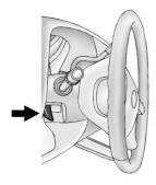
For vehicles with a tilt steering wheel, the lever is located on the left side of the steering column.
