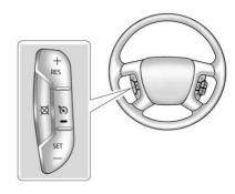
: Press to turn cruise control on or off. The white indicator comes on in the instrument cluster when cruise control is turned on.
