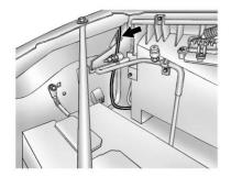
Connect the other end of the negative (-) cable to the negative (-) terminal location on the vehicle with the dead battery. On your van, use the unpainted radio antenna bracket as a remote negative (-) terminal.
