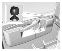
If equipped with power mirrors, select each mirror by turning the knob clockwise for the passenger side mirror or counterclockwise for the driver side mirror. The center position is neutral.
