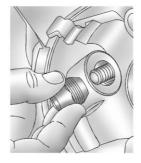
Put the wheel nuts back on with the rounded end of the nuts toward the wheel. Tighten each wheel nut by hand until the wheel is held against the hub.  Turn the jack handle counterclockwise to lower the vehicle. Lower the jack completely.
