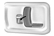
To open the front portion of a 60/40 door from the inside, pull the handle toward you and push the door open.
