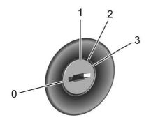
The ignition switch has four different positions.
