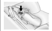
Remove the retaining wing bolt and lift it out of the mounting bracket to access the equipment.
