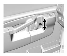
To lock the door from the inside, slide the manual lever on the door down. To unlock the door, slide the manual lever up.
