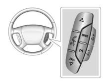
If equipped with audio steering wheel controls, some audio controls can be adjusted at the steering wheel.
