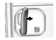
To open the sliding side door from the inside, pull the handle toward the rear of the vehicle. Then, slide the door toward the rear of the vehicle.
