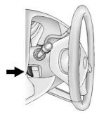
If equipped with a tilt steering wheel, the lever is on the left side of the steering column.
