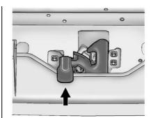
Go to the front of the vehicle and lift up the secondary hood release, which is underneath the middle of the hood.
