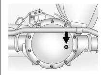
For axles with the fill plug located on the back cover of the rear axle, the proper level is 15 mm to 40 mm (0.59 to 1.57 in) below the bottom of the fill hole.
