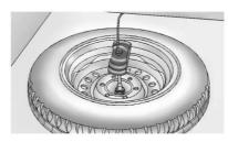
When the tire has been lowered, pull it closer to reach the tire retainer and pull it up through the wheel opening.
