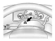
🛆: Press this button to make the front and rear turn signal lamps flash on and off. This warns others that you are having trouble. Press again to turn the flashers off.
