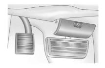
To set the parking brake, hold the regular brake pedal, then push down the parking brake pedal.
