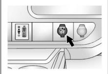
If equipped, the USB port is on the instrument panel and uses the USB 2.0 standard.
