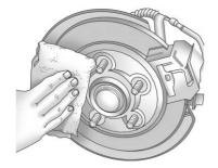
8. Remove any rust or dirt from the wheel bolts, mounting surfaces, and spare wheel.
