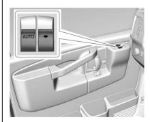
If equipped with power windows, press or pull up on the switch to lower or raise the window. The driver door also has a control to operate the front passenger window.
