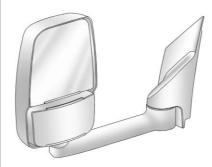
Vehicles with towing mirrors can be adjusted manually for a clear view of the objects behind you.
