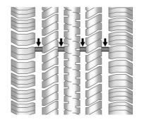
Treadwear indicators are one way to tell when it is time for new tires. Treadwear indicators appear when the tires have only 1.6 mm (1/16 in) or less of tread remaining.
