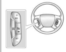
Press to turn cruise control on or off. The white indicator comes on in the instrument cluster when cruise control is turned on.
