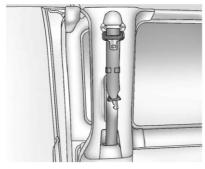
For the second and third row seats, stow the safety belt latch by attaching the clip on the safety belt latch to the trim just inside the side door.
