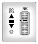
**AUX:** The thumbwheel for this system is on the instrument panel below the audio system.
