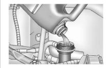
3. Fill the radiator with the proper DEX-COOL coolant mixture, up to the base of the filler neck. See Recommended Fluids and Lubricants
