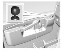
If equipped with power mirrors, select each mirror by turning the knob clockwise for the passenger side mirror or counterclockwise for the driver side mirror. Adjust the mirror angle by moving the knob in the desired direction.
