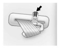
For the last row of seats, stow the safety belt latch plate on the clip at the window trim. Roll the mini-latch into the safety belt webbing and then hook the safety belt latch plate on the clip.
