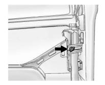
Remove the retaining wing bolt and lift it off of the mounting bracket.
