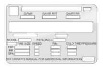
A vehicle specific Certification/ Tire label is attached to the center pillar (B-pillar). The label may show the size of the vehicle's original tires and the inflation pressures needed to obtain the gross weight capacity of the vehicle. This is called Gross Vehicle Weight Rating (GVWR). The GVWR includes the weight of the vehicle, all occupants, fuel, and cargo.
