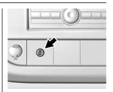
Press ♣ on the instrument panel once to turn off the TCS. The appropriate message is displayed in the DIC. See *Ride Control System Messages* \$\phi\$ 116.
