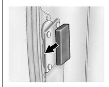
To open the rear portion of a 60/40 door from the outside, pull the handle on the side of the rear door and pull the door toward you.
