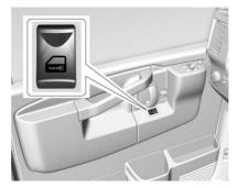
If equipped, press **a** to lock or unlock the doors.
