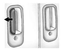
To open the sliding side door from the outside, pull the handle toward the rear of the vehicle and slide the door open.
