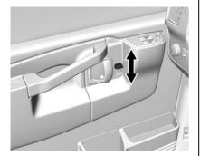
Lock and unlock the door from the outside using the key or the Remote Keyless Entry (RKE) transmitter, if equipped. From the inside, slide the manual lever on the door up or down.
