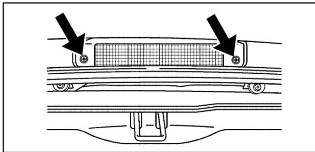
1. Remove the two screws from the CHMSL assembly.
