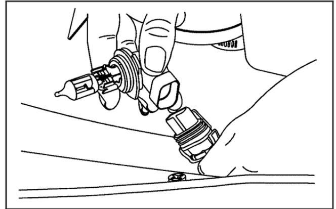
12. Install the new bulb into the socket then reinstall it into the headlamp assembly.
