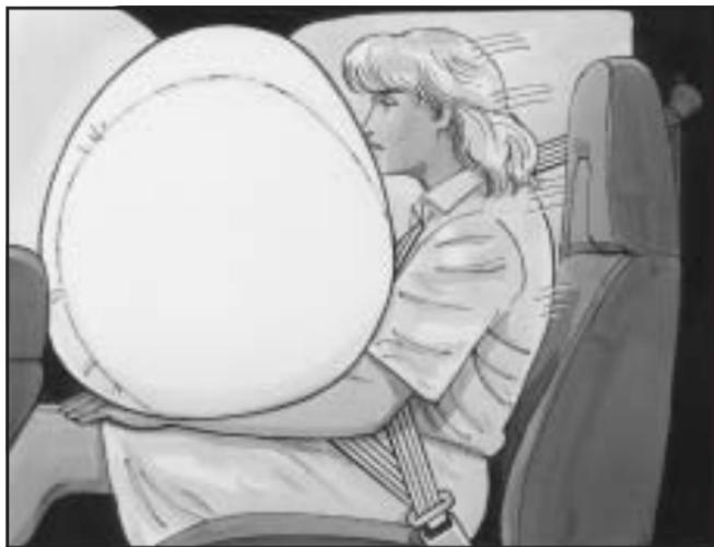
If your vehicle has one, the right front passenger's airbag is in the instrument panel on the passenger's side.
