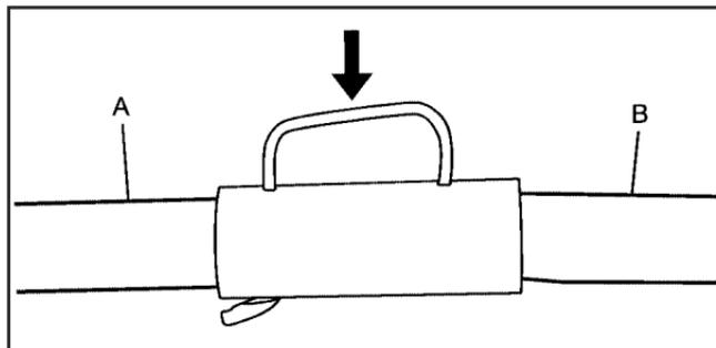
3. Connect the jack handle (A) and jack handle extension (B) together and press the retention clip (arrow) so it engages.
