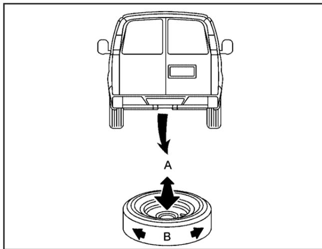
7. Make sure the tire is stored securely. Push, pull (A), and then try to turn (B) the tire. If the tire moves, use the ratchet to tighten the cable.
