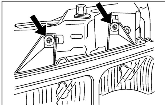
3. Remove the two pins on the top of the headlamp assembly. To remove the pins, turn the outer pin clockwise and pull it straight up. To remove the inner pin, turn it counterclockwise and pull it straight up.
