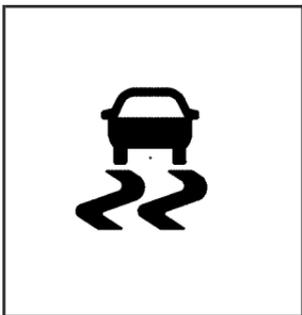
Pressing and holding the StabiliTrak<sup>®</sup> button located on the instrument panel for more than five seconds can turn off StabiliTrak<sup>®</sup> and part of the traction control system.
