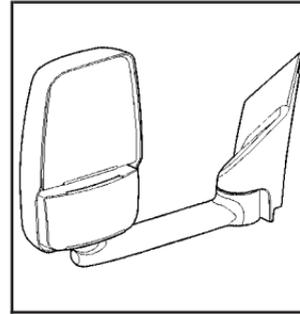
If your vehicle has these camper-type mirrors, they can be adjusted manually so you can have a clear view of the objects behind you.
