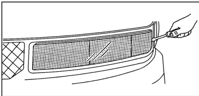
1. Use a small tool to unlatch the outboard clip on the lamp.
