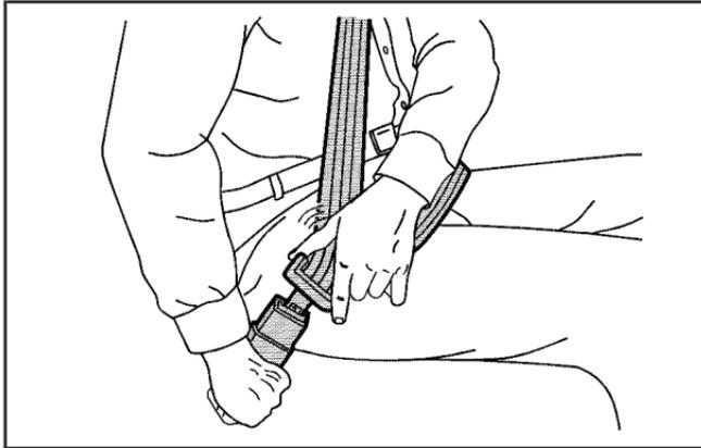
3. Push the latch plate into the buckle until it clicks. Pull up on the latch plate to make sure it is secure. If the belt is not long enough, see *Safety Belt Extender* on page 1-28.
