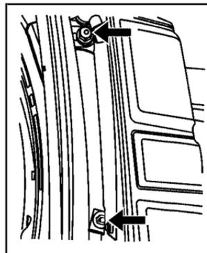
1. Remove the two inboard nuts from the inside of the taillamp assembly.
