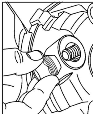
9. Put the wheel nuts back on with the rounded end of the nuts toward the wheel. Tighten each wheel nut by hand until the wheel is held against the hub.
