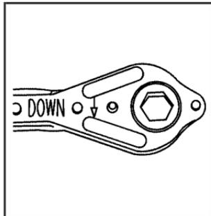
1. Attach the wheel wrench and ratchet, with the DOWN side facing you. The wheel wrench has a socket end and a flat chisel end. Note that there is an UP side and a DOWN side on the ratchet.
