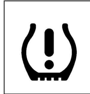
When a low tire pressure condition is detected, the TPMS will illuminate the low tire pressure warning symbol located on the instrument panel cluster.
