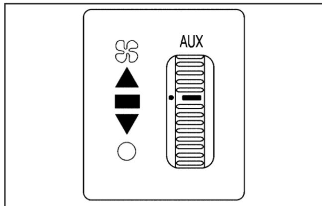
**AUX:** The thumbwheel for this system is located in the switchbank below the audio system.
