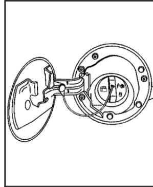
The tethered fuel cap is located behind a hinged fuel door on the driver side of the vehicle.
