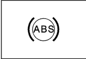
With the Anti-Lock Brake System (ABS), this light will come on when the engine is started and may stay on for several seconds.
