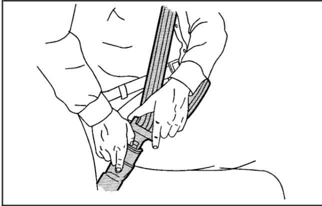
To unfasten the belt, push the button on the buckle. The belt should go back out of the way.
