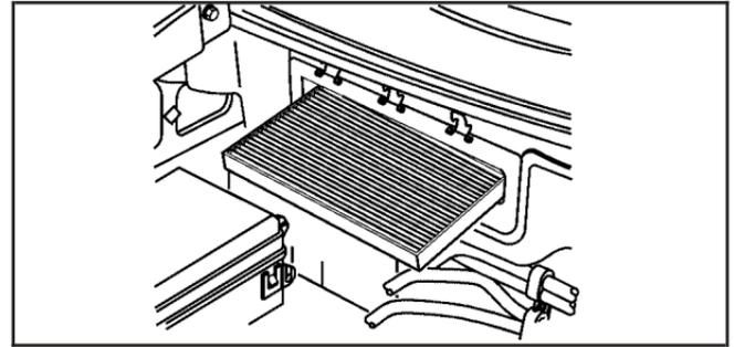
3. Remove the passenger compartment air filter from the housing.
