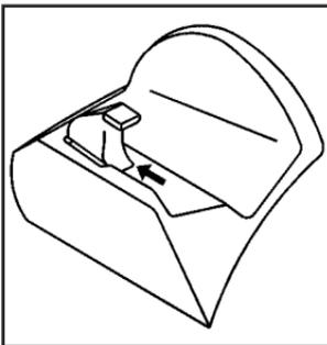
2. Insert the roof panel so that the outside front edges line up between the receiver covers. Push forward on the roof panel until it stops.
