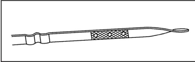
If the oil is below the cross-hatched area at the tip of the dipstick, you will need to add at least one quart/liter of oil. But you must use the right kind. This section explains what kind of oil to use. For engine oil crankcase capacity, see *Capacities and Specifications on page 427*.
