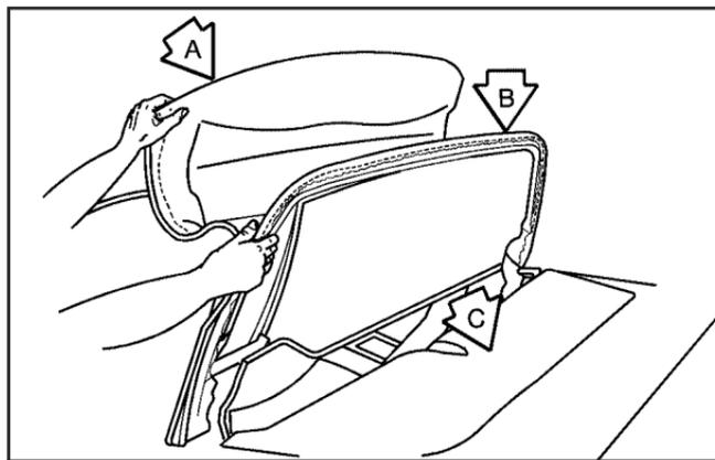
5. Lift upward on the front edge (A) of the convertible top off of the windshield frame. Then lift upward on the rear edge (B) of the convertible top so it is vertical to the tonneau cover (C). The front edge (A) and rear edge (B) should be straight up.
