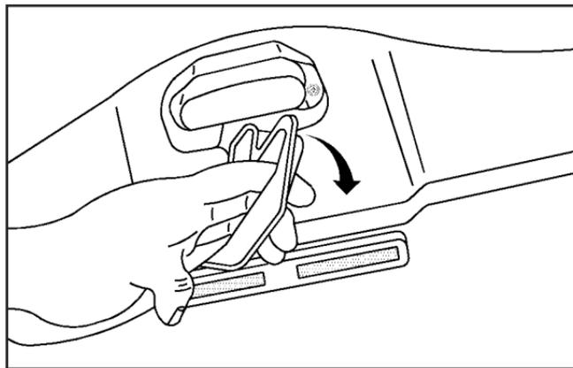
3. Release the convertible top front latch, located above the inside rearview mirror, by pulling and turning it clockwise toward the driver's door. Push upward on the front edge. The windows will automatically lower.
