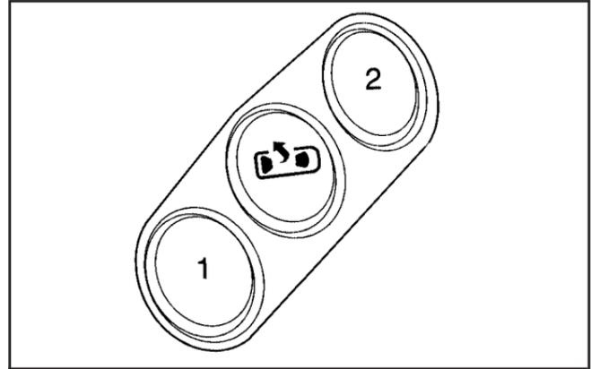
If your vehicle has this feature, memory can program and recall the settings for the driver's seating position. The controls for this feature are located on the driver's door.
