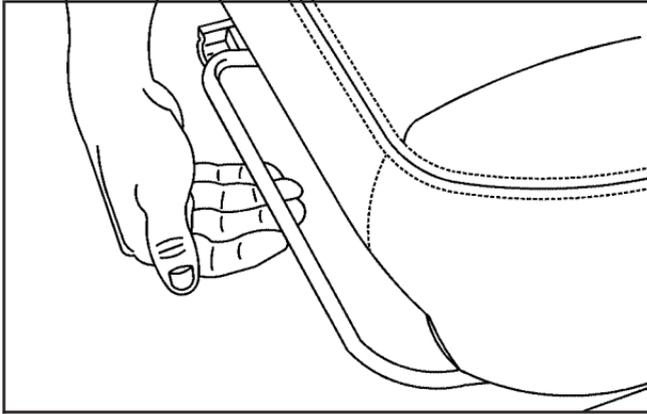
To move a manual passenger seat, pull up the bar located under the front of the seat to unlock it. Slide the seat to where you want it and release the bar. Then try to move the seat forward with your body to make sure it is locked into place.
