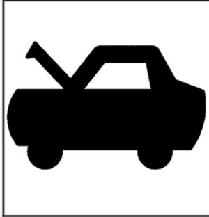
1. Pull the hood release lever with this symbol on it. It is located inside the vehicle below the instrument panel on the driver's side.
