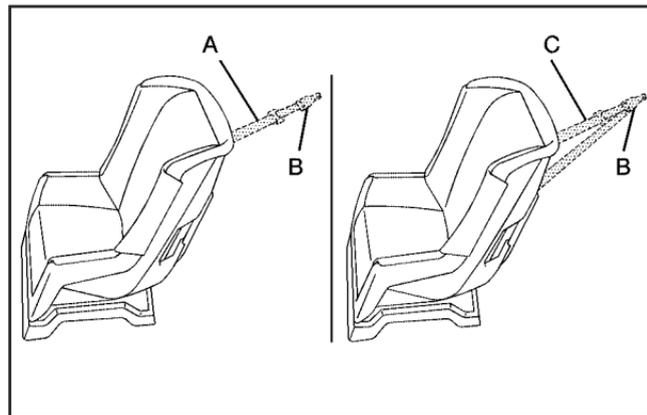
A top tether (A, C) anchors the top of the child restraint to the vehicle. A top tether anchor is built into the vehicle.
