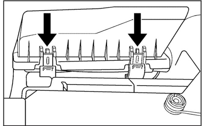
1. Pull the latches on each side of the cover to open, then move the latches up and out of the way.
