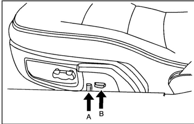
Your vehicle may have power lumbar and side bolsters. The switches are located on the outboard side of the seat cushion.
