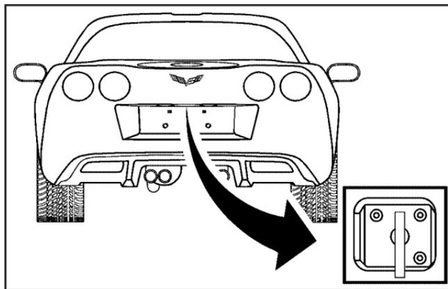
If your vehicle has lost battery power, open the hatch/trunk using the vehicle key located inside the keyless access transmitter. See *Keys on page 71* for more information. The key lock cylinder is located on the rear of the hatch/trunk lid above the license plate. Turn the vehicle key clockwise in the lock.
