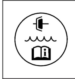
The hydraulic clutch fluid reservoir cap has this symbol on it. See *Engine Compartment Overview on page 328* for reservoir location.
