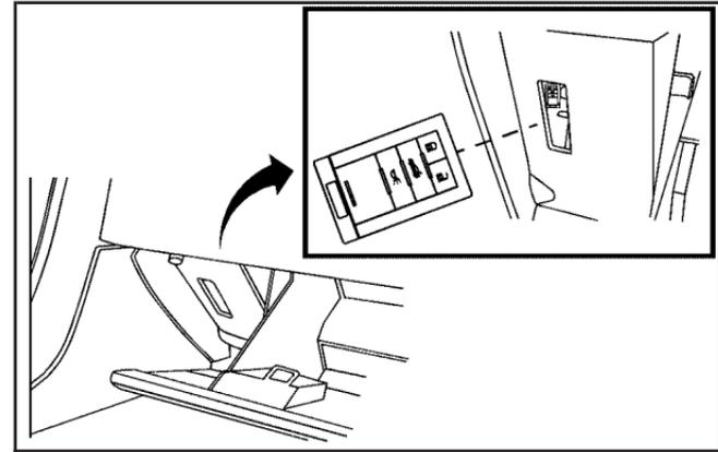
7. Place the new, unrecognized transmitter in the glove box transmitter pocket with the buttons facing towards the passenger's side.
