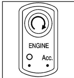
Your vehicle has an electronic keyless ignition with a pushbutton start.
