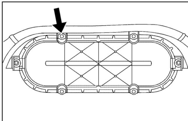
1. Remove the screws holding the filter element in place.
