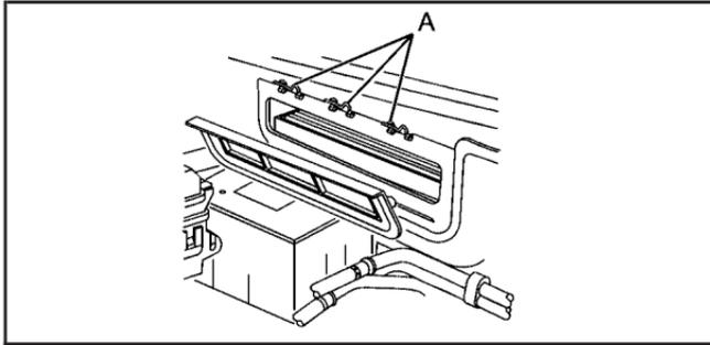
1. Undo the passenger compartment air filter housing cover retainer clips (A).
