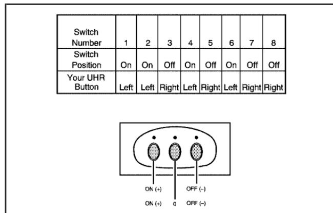
4. The indicator light will blink slowly. In order from left to right, and within two and one-half minutes, enter each switch setting into the Universal Home Remote System. Push one button for each switch as follows:
