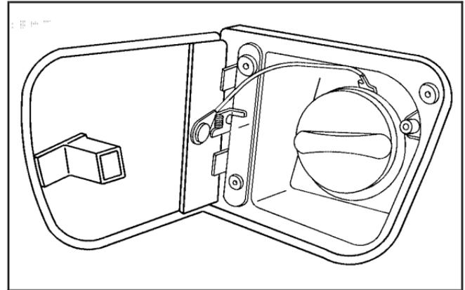
The tethered fuel cap is located behind a hinged fuel door on the driver's side of the vehicle.
