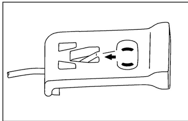
From outside the vehicle, use the key in the cylinder above the license plate to open the hatch. Use the door release tab located on the carpet inside the trunk on the driver's side of the vehicle. Pull the tab to unlock and unlatch the driver's door. See *Keys* on page 71 for information on opening the trunk during a loss of power.
