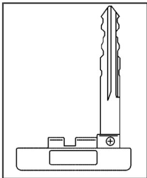
There is a key, located inside the keyless access transmitter, that works the glove box and can open the hatch/trunk lid if vehicle power is lost. See *Hatch/Trunk* on page 83 for more information.
