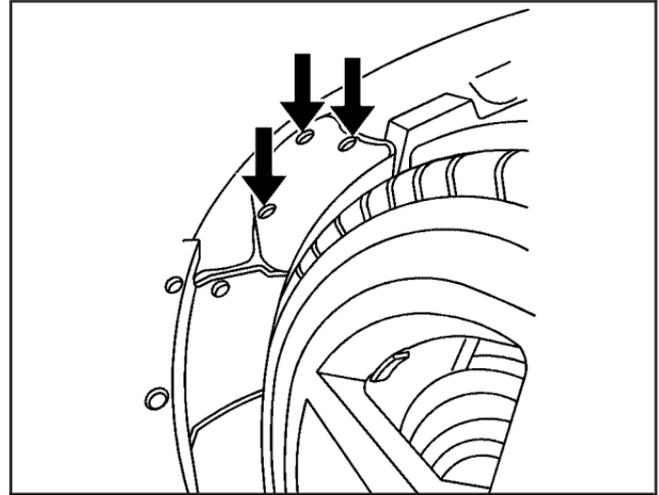
2. Access the high-beam or front parking/turn signal bulbs by removing the access panel. To do this, remove the three outer fasteners and move the cover back.
