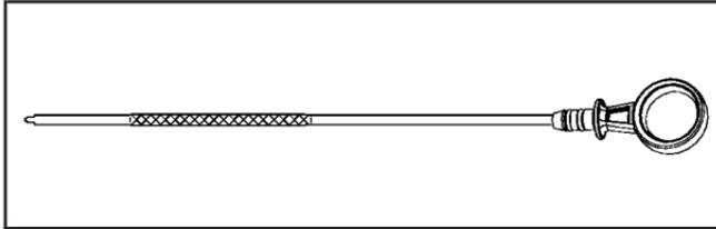
If the oil is below the cross-hatched area at the tip of the dipstick, you will need to add at least one quart/liter of oil through the oil fill cap opening in the oil tank. But you must use the right kind. This section explains what kind of oil to use. For engine oil crankcase capacity, see *Capacities and Specifications on page 427*.
