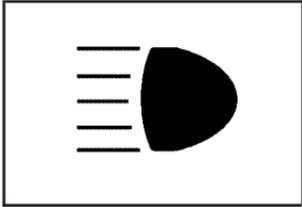
While the high beams are on, this light on the instrument panel cluster will also be lit.
