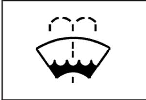
Open the cap with the washer symbol on it. Add washer fluid until the tank is full. See *Engine Compartment Overview* on page 328 for reservoir location.
