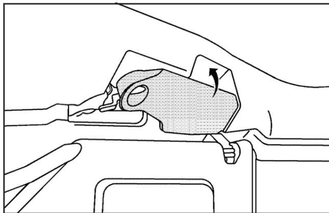
**Driver's Side Front Roof Panel Release Latch**
