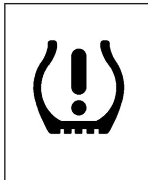
As an added safety feature, your vehicle has been equipped with a tire pressure monitoring system (TPMS) that illuminates a low tire pressure telltale when one or more of your tires is significantly under-inflated.
