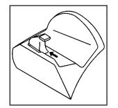
2. Insert the roof panel so that the outside front edges line up between the receiver covers. Push forward on the roof panel until it stops.
