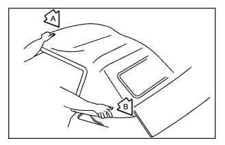
8. Push forward on the front edge (A) of the convertible top to allow the rear edge (B) of the convertible top to be moved to its full-down position.
