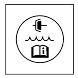
The hydraulic clutch fluid reservoir cap has this symbol on it. See *Engine Compartment Overview* on page 5-12 for reservoir location.
