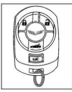
Your vehicle comes standard with two transmitters, and up to four can be matched to your vehicle. See "Matching Transmitter(s) to Your Vehicle" later in this section.
