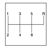
This is the shift pattern for the six-speed manual transmission.
