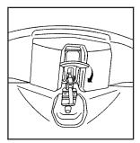
Push up on the handle of the rear roof release handle to latch its hook in the closed position.
