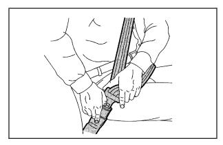
To unlatch the belt, just push the button on the buckle. The belt should go back out of the way.
