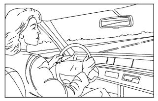
An emergency like this requires close attention and a quick decision. If you are holding the steering wheel at the recommended 9 and 3 o'clock positions, you can turn it a full 180 degrees very quickly without removing either hand. But you have to act fast, steer quickly, and just as quickly straighten the wheel once you have avoided the object.
