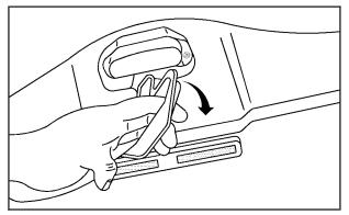
4. The convertible top front latch, located above the inside rearview mirror, must be unlocked. Pull the convertible top front latch down and turn it clockwise to unlock it.
