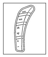
The HUD controls are located to the left of the steering wheel.
