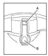
To unlock the rear of the roof panel's rear release latch, press the back of the release handle (B). Then press the button on the front of the release handle, (A) with your thumb.
