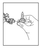
Remove the headlamp bulb by releasing the outer tabs from the socket.
