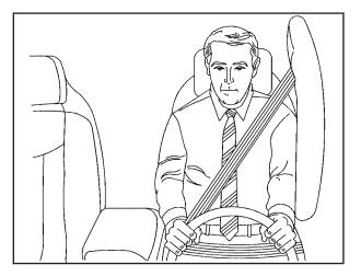
If your vehicle has a side impact airbag for the driver, it is in the side of the driver's seatback closest to the door.
