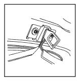
Push the loop to the top of the striker (base plate).
