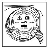
The engine coolant surge tank is located toward the rear of the engine compartment on the driver's side of the vehicle. See Engine Compartment Overview on page 5-12 for more information on location.
