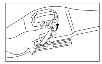
11. Pull the top front latch handle down and turn it counterclockwise to lock the convertible top.
