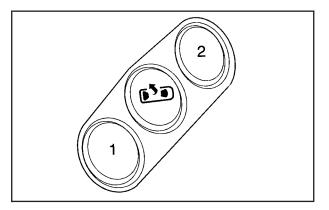
If your vehicle has this feature, memory can program and recall the settings for the driver's seating position. The controls for this feature are located on the driver's door. The numbers on the back of the keyless access transmitters, 1 and 2, correspond to the numbers on the memory buttons.
