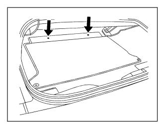
To install the rear trunk partition, secure the partition onto the retainers located on the floor of the trunk towards the front of the compartment.
