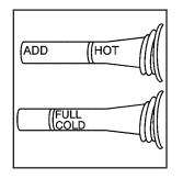
When the engine compartment is hot, the level should be at the HOT mark. When the engine compartment is cool, the level should be at the FULL COLD mark.
