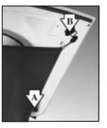
Hook the elastic loops on the front corners (A) of the shade to the T-nuts located on the front corners of the rear hatch frame.
