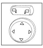
The controls for the outside power mirrors are located on the driver's door.
