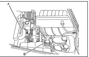
A. Electric Engine Cooling Fan
