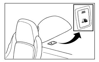
The top tether anchor is located behind the passenger seat.
