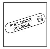
There is also a manual fuel door release tab. It is located against the upper trim in the rear compartment on the driver's side of the vehicle. Pull the tab to release the fuel door.
