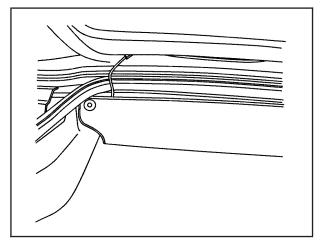
Pull the divider up and snap it onto the snaps on both sides of the trunk.
