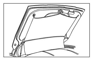
3. Grasp the loop at the rear center of the shade and wrap around the striker assembly.
