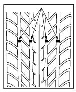
One way to tell when it is time for new tires is to check the treadwear indicators, which will appear when your tires have only 1/16 inch (1.6 mm) or less of tread remaining. You need a new tire if any of the following statements are true:
