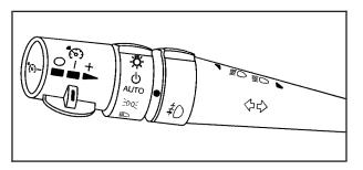
The exterior lamp control is located to the left of the steering wheel on the multifunction lever.
