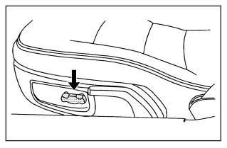
The control for the driver's power seat is located on the outboard side of the seat cushion. Your vehicle may also have a passenger power seat.
