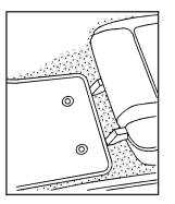
To remove the floor mats, pull up on the rear of the mat to disconnect from the locator pins.
