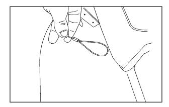
7. Pull the cable to release the tonneau cover.
