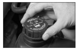
You can remove the coolant surge tank pressure cap when the cooling system, including the coolant surge tank pressure cap and upper radiator hose, is no longer hot. Turn the pressure cap slowly counterclockwise about one-quarter turn and then stop.
