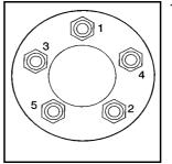
13. Tighten the wheel nuts firmly in a crisscross sequence, as shown.
