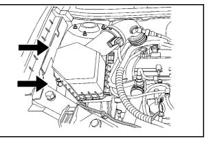
5. To remove the filter cover, unlatch the clamps, then pull up on the front and pull out.
