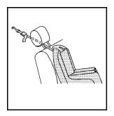
If the position you are using has an adjustable headrest or head restraint and you are using a single tether, raise the headrest or head restraint and route the tether under the headrest or head restraint and in between the headrest or head restraint posts. 3. Push and pull the child restraint in different directions to be sure it is secure.
