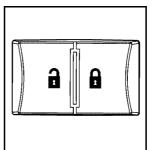
This vehicle may have power door locks. The controls are located on the driver and front passenger door armrests.
