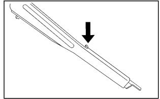
Press the button and then pull on the end of the wheel wrench to extend the handle.
