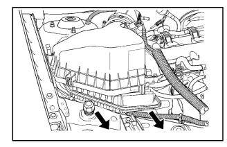
6. Remove filter and inspect or replace.
