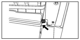
2. Lower the glove box door by pressing in on each side and lowering from the track.
