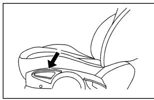
To raise or lower the driver seat, move the lever upward or downward repeatedly until the seat is at the desired height.
