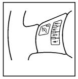
The cruise control buttons are located on the outboard side of the steering wheel.
