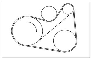
Dotted line shows routing for vehicles without air conditioning.
