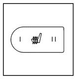
Press the side of the switch with the double indicator lights to turn on the heated seat at the highest setting.
