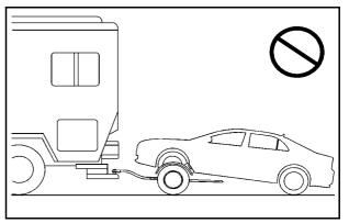
*Notice:* Towing the vehicle from the rear could damage it. Also, repairs would not be covered by the vehicle warranty. Never have the vehicle towed from the rear.
