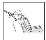
If the position you are using has a fixed or adjustable headrest or head restraint and you are using a dual tether, route the tether around the headrest or head restraint.
