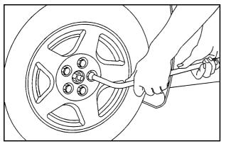
3. If necessary, use the flat end of the wheel wrench to pry along the edge of the wheel cover until it comes off.
