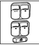
For vehicles with power windows, the switches on the driver door armrest control each window. The switch on each passenger door controls only that doors window. Press the front of the switch to open the window and pull the switch up to close it.
