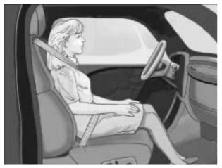
If a person of adult-size is sitting in the right front passenger seat, but the off indicator is lit, it could be because that person is not sitting properly in the seat. If this happens, use the following steps to allow the system to detect that person and enable the right front passenger frontal airbag:
