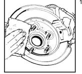
10. Remove any rust or dirt from the wheel bolts, mounting surfaces, and spare wheel.
