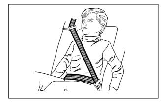
4. Buckle, position, and release the safety belt as described previously in this section. Make sure that the shoulder belt crosses the shoulder.
