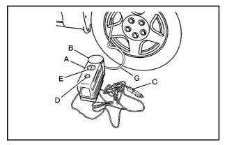
When using the tire sealant and compressor kit during cold temperatures, warm the kit in a heated environment for 5 minutes. This will help to inflate the tire faster. Always do a safety check first. See *If a Tire Goes Flat on page 6-82*. Do not remove any objects that have penetrated the tire.
