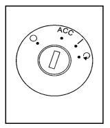
The ignition switch has four different positions.
