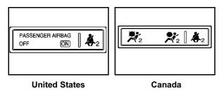
The words ON and OFF, or the symbol for on and off, will be visible during the system check. If you are using remote start to start the vehicle from a distance, if equipped, you may not see the system check. When the system check is complete, either the word ON or the word OFF, or the symbol for on or off, will be visible. See *Passenger Airbag Status Indicator on page 4-22*.
