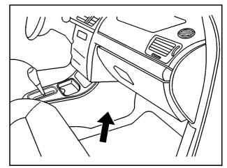
The floor console fuse block is located on the passenger side of the floor console behind the forward panel. The panel has three clips. Pull the panel to disconnect the three clips, and access the fuses. Use the fuse puller to remove fuses.
