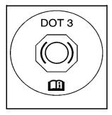
The brake master cylinder and, on manual transmission vehicles, the clutch hydraulic system use the same reservoir filled with DOT 3 brake fluid.
