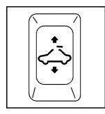
On vehicles with a sunroof, the switch that operates it is located on the headliner between the map lamps.
