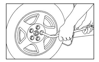
2. If your vehicle has plastic wheel covers, use the wheel wrench to loosen the plastic wheel nut caps.
