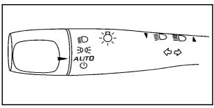
The lever on the left side of the steering column operates the exterior lamps.
