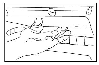
3. Pull the tab at the back of the glove box toward you and open the passenger compartment air filter door downward.
