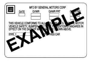
A vehicle specific Certification label, found on the rear edge of the driver door, tells you the gross weight capacity of your vehicle, called the Gross Vehicle Weight Rating (GVWR). The GVWR includes the weight of the vehicle, all occupants, fuel, and cargo. Never exceed the GVWR for your vehicle, or the Gross Axle Weight Rating (GAWR) for either the front or rear axle.
