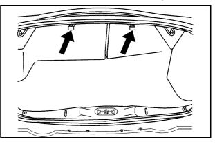
1. Open the trunk and pull one or both of the small handles located in the center of the trunk.
