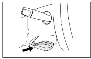
The tilt wheel lever is located on the left side of the steering column.
