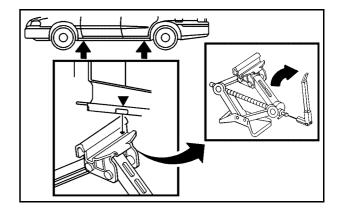
Position the jack lift head at the rear jack location nearest the rear tire. The rear location is about 4 inches (10 cm) in front of the rear wheel opening.
