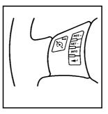
The cruise control buttons are located on the left side of the steering wheel.
