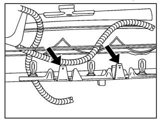
3. Pull the bulb assembly down to access the bulbs.
