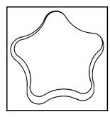
If equipped, the lumbar knob is located on the front of the driver seat lower cushion. Turn it clockwise or counterclockwise to increase or decrease the lumbar support.
