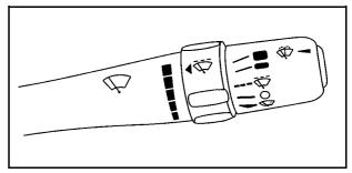
To change the headlamps from high beam to low beam, pull the turn signal lever toward you.
