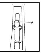
Press the release button (A) and move the height adjuster to the desired position. The adjuster can be moved up by pushing up on the shoulder belt guide.
