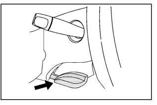
The tilt wheel lever is located on the left side of the steering column.
