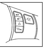
If equipped, some audio controls can be adjusted using the controls on the right side of the steering wheel.
