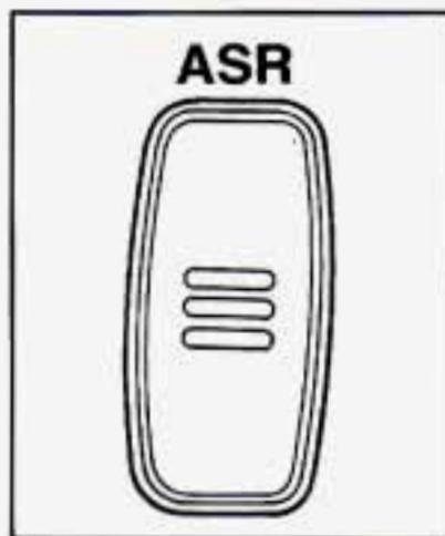
To turn the system off, press the button on the console near the cigarette lighter.
