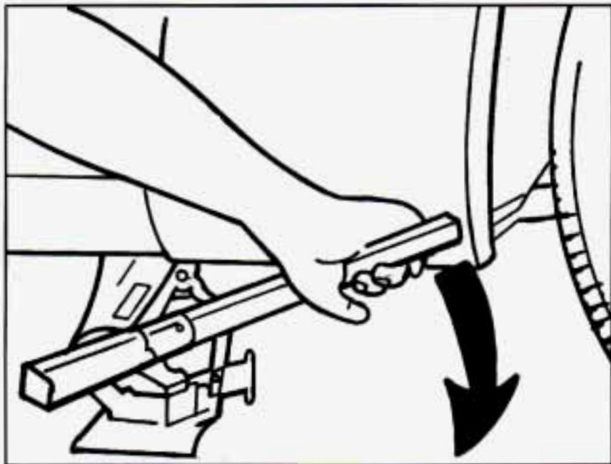
3. Raise the vehicle by rotating the wheel wrench clockwise. Raise the vehicle far enough off the ground so there is enough room for the spare tire to fit.
