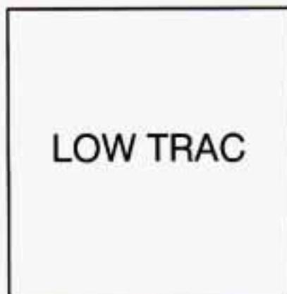
When your anti-lock system is adjusting brake pressure to help avoid a braking skid, this light will come on.
