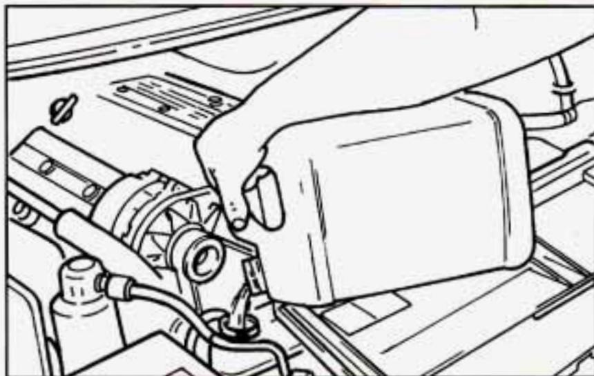
4. Fill with the proper mix. Add coolant until you see a steady stream of coolant coming from the bleed valves.
