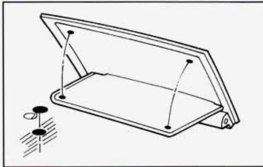
5. Pull the sunshade back a little and remove the backing paper from the velcro buttons. Push the sunshade back into place, sticking the velcro to the glass.
