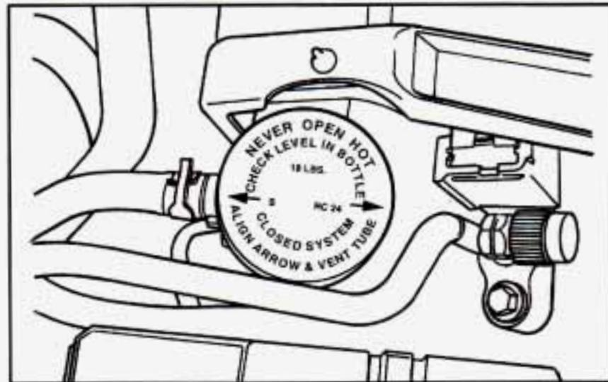
8. Then replace the pressure cap. At any time during this procedure if coolant begins to flow out of the filler neck, reinstall the pressure cap. Be sure the arrows on the pressure cap line up like this.
