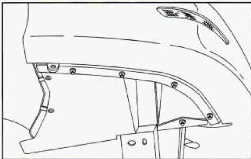
1. Using a screwdriver, remove the plastic screws from the deflector under the vehicle. Move the deflector out of the way.
