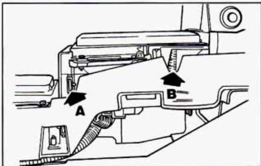
9. Check the headlamp aim indicators. The horizontal indicator (A) should be on 0 (zero). If the vehicle is level, the vertical indicator (B) should also be on 0 (zero). If the vehicle isn't level, check the vertical aim on a level surface as soon as you can. If either indicator doesn't read 0 (zero), adjust the headlamp aim. See "Adjusting Headlamp Aim" in the Index.
