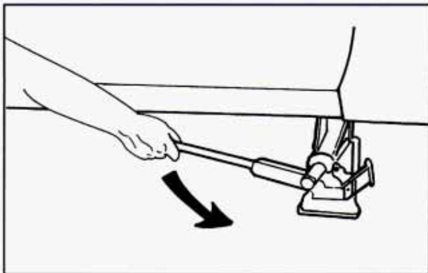
5. Lower the vehicle by rotating the wheel wrench counterclockwise. Lower the jack completely.
