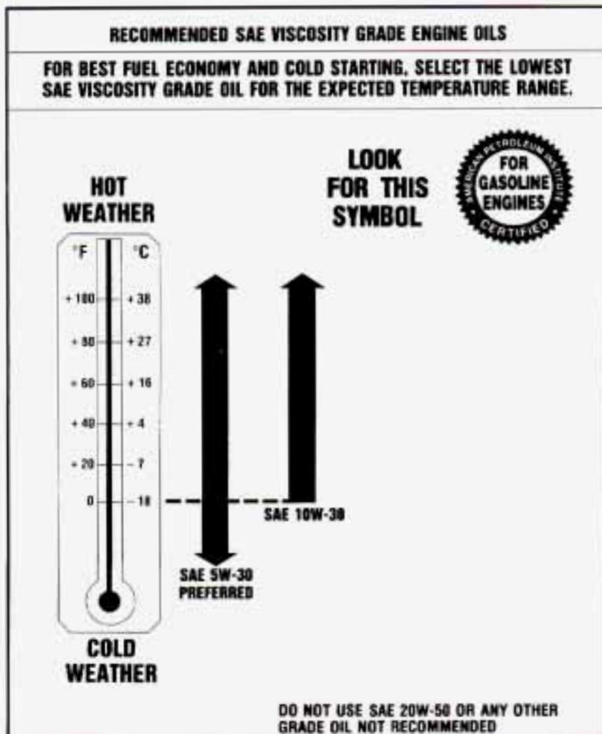
As shown in the chart, unless you have the 3.8L engine, SAE 5W-30 is best for your vehicle. However, you can use SAE 10W-30 if it's going to be 0°F (-18°C) or above. These numbers on an oil container show its viscosity, or thickness. Do not use other viscosity oils, such as SAE 20W-50.
