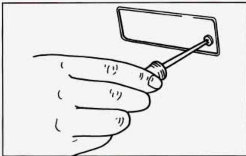
Replacing a rear sidemarker bulb:
