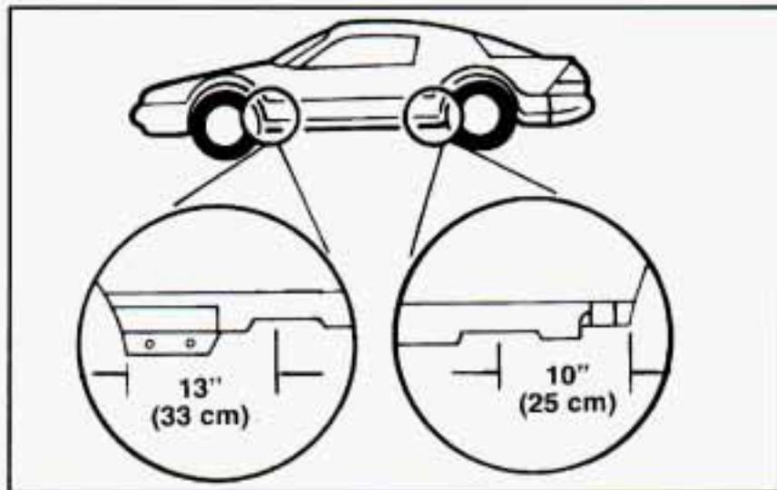
2. Position the jack under the vehicle. There is a notch in the vehicle's rocker flange. Raise the jack head until it fits firmly into the notch nearest the flat tire.
