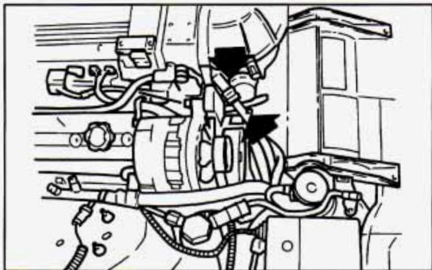
3. After the engine cools, open the air bleed valves on the heater return hose and water pump inlet.
