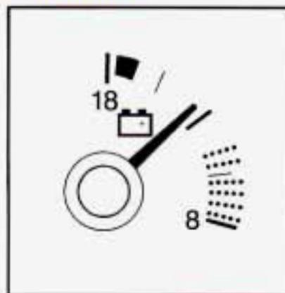
You can read battery voltage on your voltmeter. If it reads less than 11 volts or more than 16 volts while your engine is running, and it stays there, you may have a problem with the electrical charging system.
