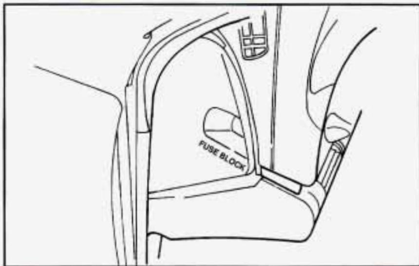
The main fuse block is located on the left side of your instrument panel. Open the cover to expose the fuses.
