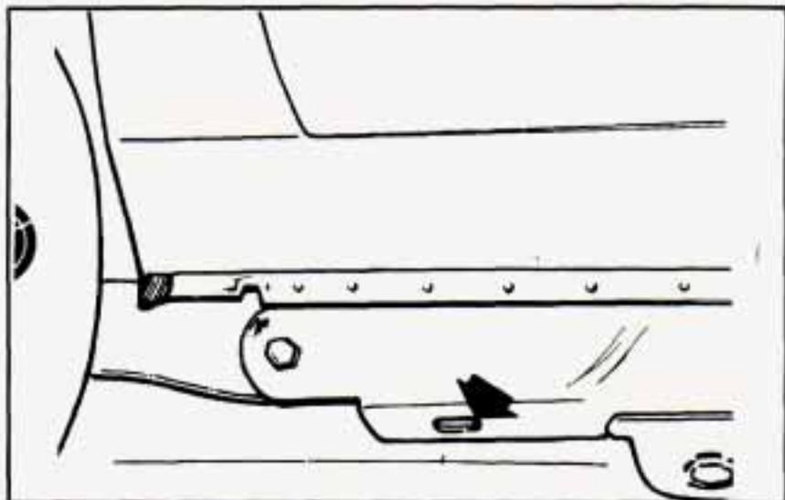
Attach T-hook chains in front of rear wheels, in the bottom of frame rail, on both sides.
