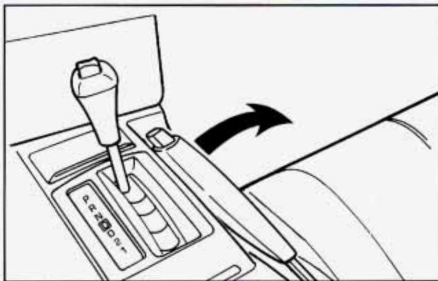
To set the parking brake, hold the brake pedal down and pull up on the parking brake lever. If the ignition is on, the brake system warning light will come on.
