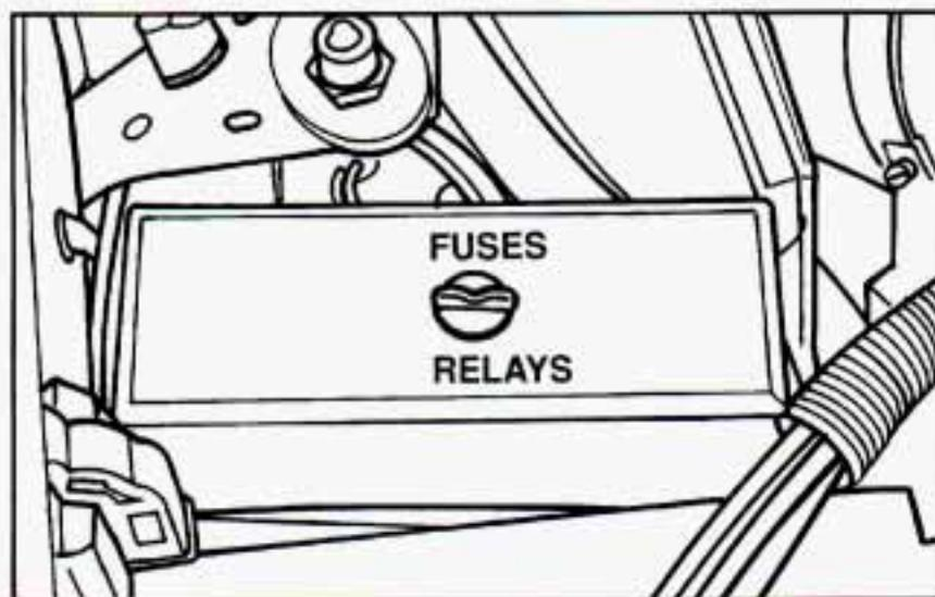
The underhood electrical center fuses are located in the engine compartment. Open the cover to expose the fuses.
