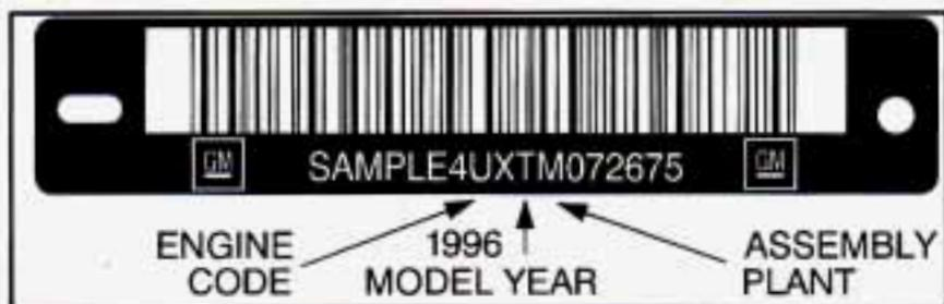
This is the legal identifier for your Chevrolet. It appears on a plate in the front corner of the instrument panel, on the driver's side. You can see it if you look through the windshield from outside your vehicle. The VIN also appears on the Vehicle Certification and Service Parts labels and the certificates of title and registration.
