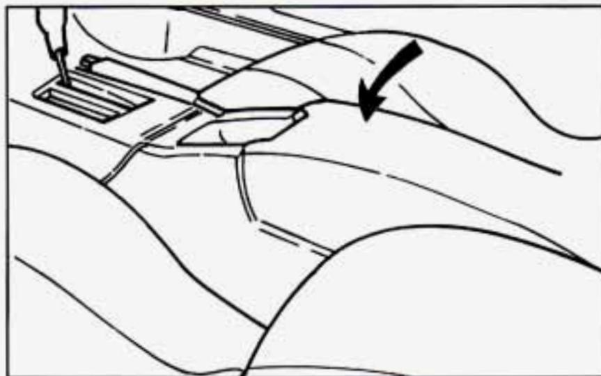
To use the storage area, pull up on the front end of the console. There is a cupholder and lamp in the console.
