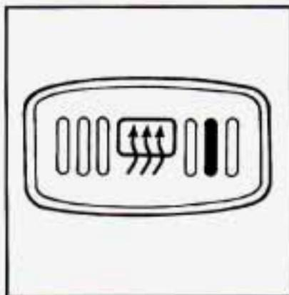
The rear window defogger uses a warming grid to remove fog from the rear window.
