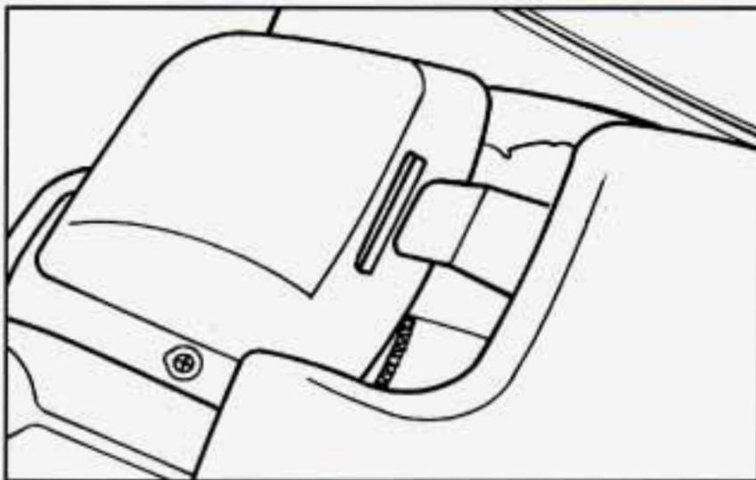
1. Open the trunk and remove the two side covers from the storage bag.
