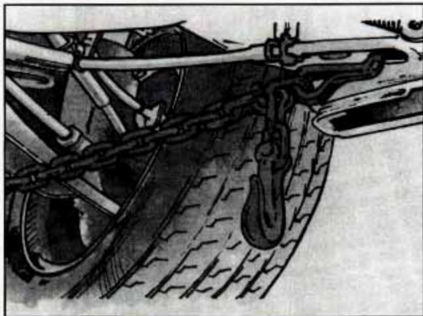
Attach T-hook chains to slots in frame, rearward of front wheels, on both sides.
