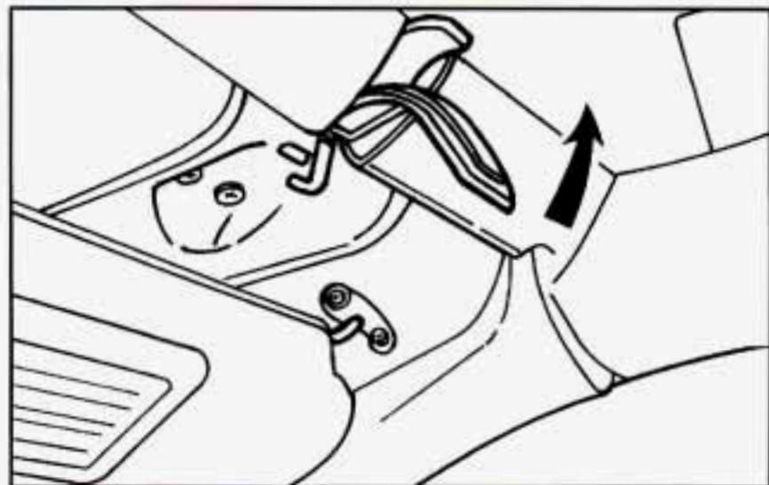
6. Pull down on the latches and align hooks with holes. Push forward on the larger part of the latch until it clicks. Do not force the latch. If it is hard to lock, the top is not properly aligned.
