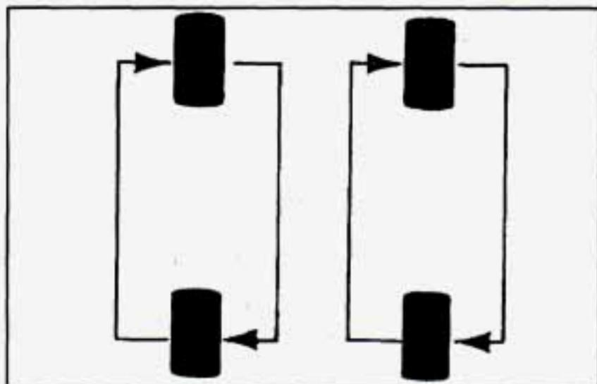
If you have P245/50ZR16 Goodyear Eagle GS-C tires, they must roll in a certain direction for the best overall performance. The direction is shown by an arrow on the sidewall. Because these tires are directional, they should be rotated as shown here. These tires should only be moved from front to rear and rear to front on the same side of the vehicle.
