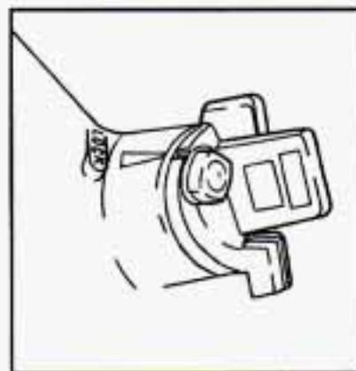
If you have a manual transmission, your ignition lock has a key release button. You must press the button before you can take your key out of the ignition lock.
