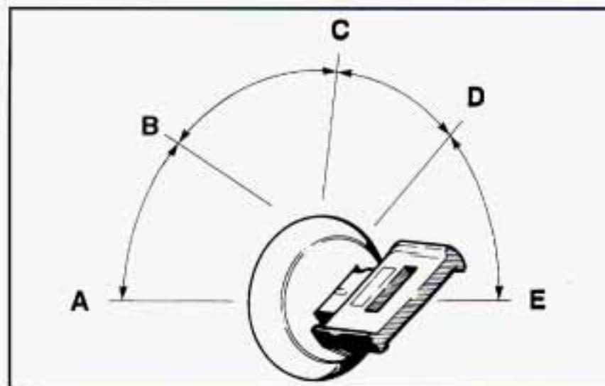
**ACC (A):** Position in which you can operate your electrical power accessories. Press in the ignition switch as you turn the top of it toward you.
