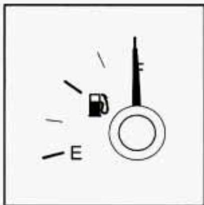
Your fuel gage shows about how much fuel is in your tank. The fuel gage works only when the ignition switch is in the RUN position.
