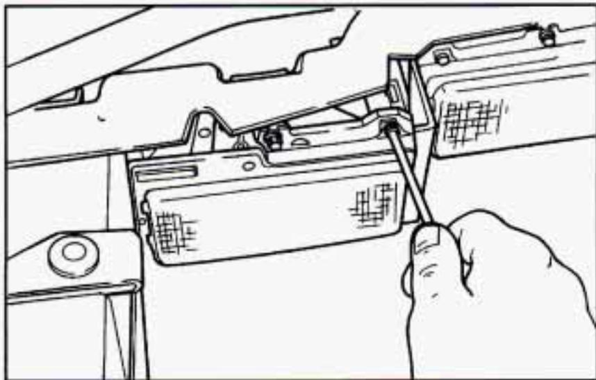
1. Remove the Torx<sup>®</sup> head screws at the end of the aiming ring.
