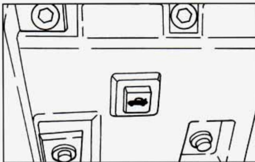
Press the switch in your glove box to unlock the hatch from inside your vehicle. If you have an automatic transmission, your shift lever must be in PARK (P) or NEUTRAL (N) to use the switch. If you have a manual transmission and the ignition switch is in RUN, you must set the parking brake before you can use the switch.
