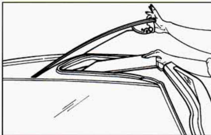
1. Start with the panel marked DRIVER FRONT. Unlatch the driver's side T-top, raise it halfway and close the latch handle.
