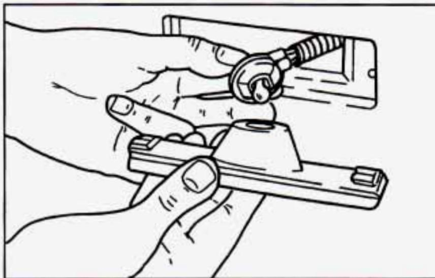
3. Turn counterclockwise and pull out the socket and the bulb.
