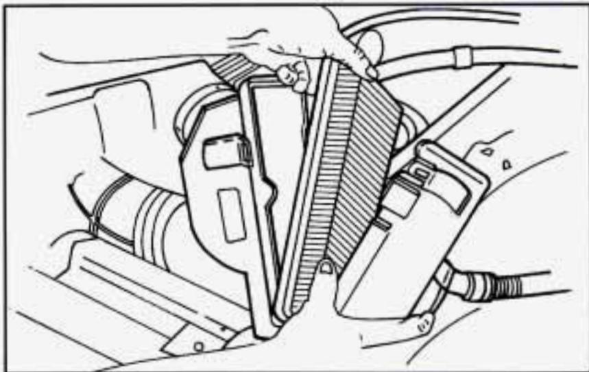
4. Open the air cleaner and remove the filter.
