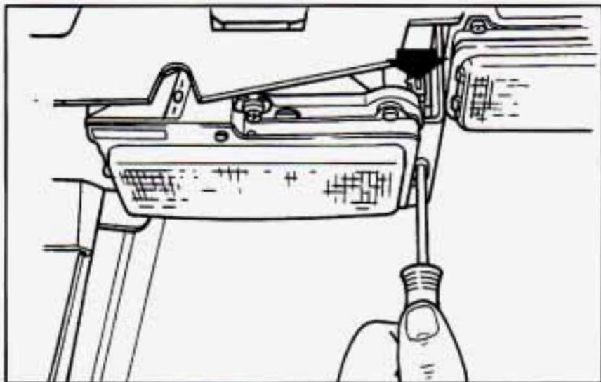
2. Start with the horizontal (left and right) headlamp aim. Don't try to adjust the vertical (up and down) aim first.
