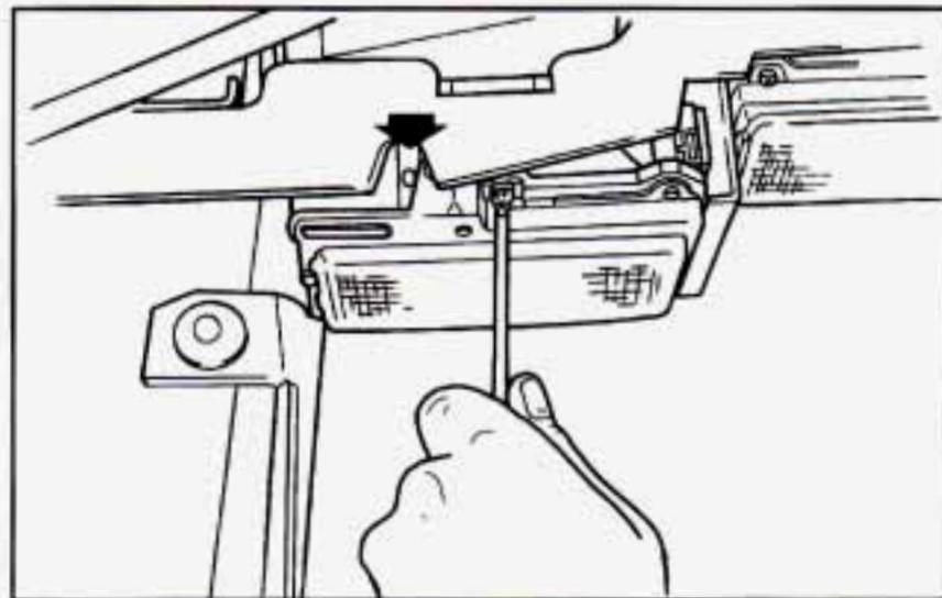
5. Now adjust the vertical aim. Check the vertical aim for each headlamp and adjust it as necessary.
