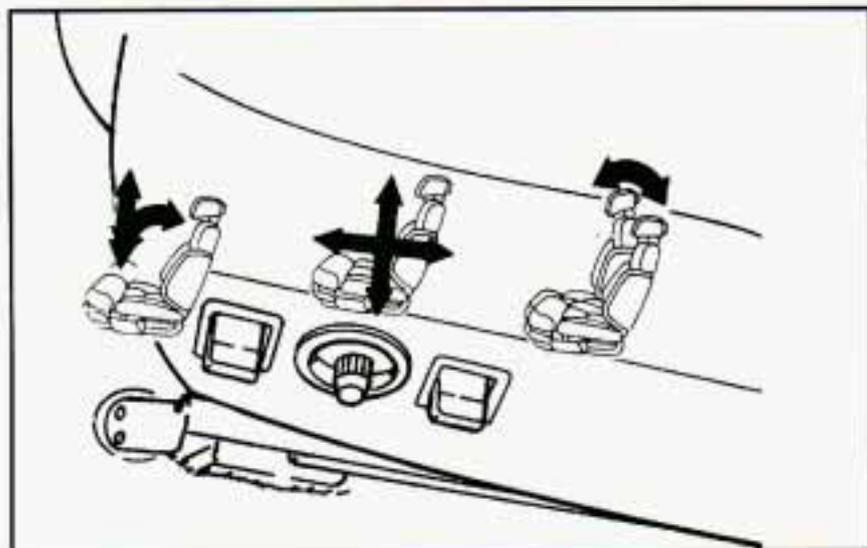
The driver's seat has three controls on the left side. The front control makes the front of the seat go up and down.
