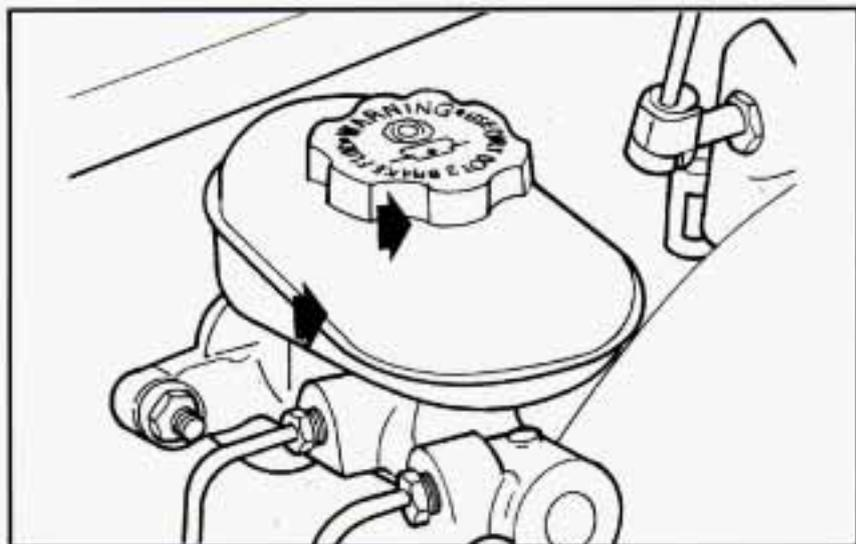
You can check the brake fluid without taking off the cap. Just look at the brake fluid reservoir. The fluid level should be above the plastic seam in the reservoir. If it isn't, have your brake system checked to see if there is a leak.
