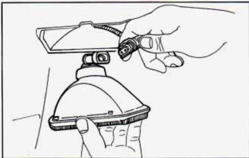
3. Pull the headlamp out of the assembly. Remove the wiring connector from the headlamp socket by lifting the plastic locking tabs on the connector and pulling it from the socket.
