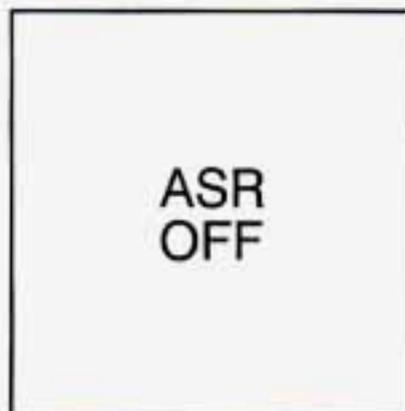
When the system is on, this warning light will come on to let you know if there's a problem with your ASR system. See "ASR System Warning Light" in the Index. When this warning light is on, the system will not limit wheel spin. Adjust your driving accordingly.
