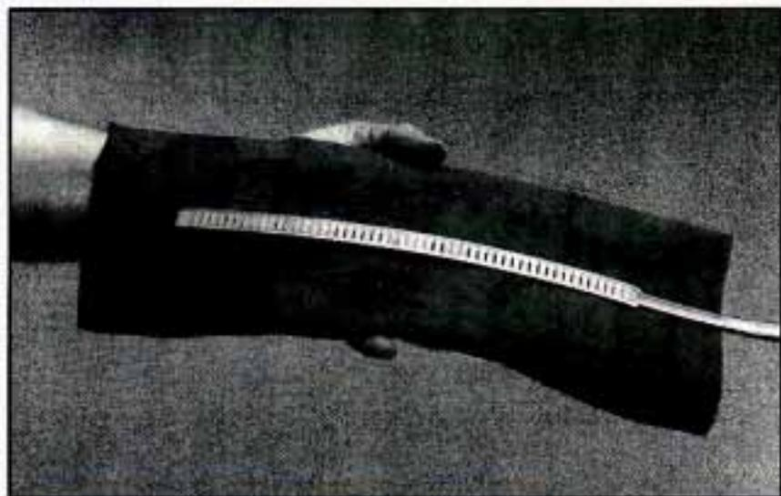
When your engine is cold, check the dipstick on the cap of the coolant recovery tank. The coolant level should be at COLD, or a little higher. When your engine is warm, the level on the dipstick should be up to HOT, or a little higher.
