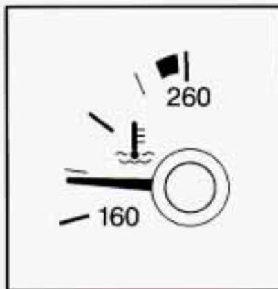
This gage shows the engine coolant temperature. If the gage pointer moves into the red area, your engine is too hot! It means that your engine coolant has overheated.
