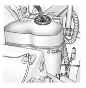
Fill the coolant surge tank with the proper mixture to the FULL COLD mark.
