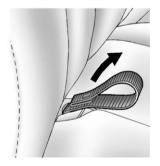
Pull the loop in the crease where the seatback and seat cushion meet to release the seat cushion. Tilt the seat cushion forward toward the front of the vehicle.
