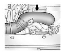
4. With the coolant surge tank pressure cap off, start the engine and let it run until the upper radiator hose can be felt getting hot. Watch out for the engine cooling fan.
