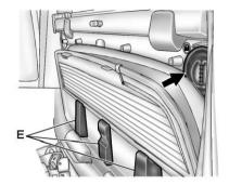
Load the rear glass into the storage pocket in the Midgate, guiding the lower edge of the rear glass behind the three rear glass retaining tabs (E).
