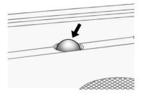
The solar sensor, located in the defrost grille, middle of the instrument panel, monitors the solar heat. Do not cover the solar sensor or the system will not work properly.
