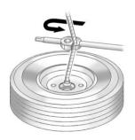
Use the wheel wrench hook to pull the hoist cable closer to assist in reaching the spare tire.
