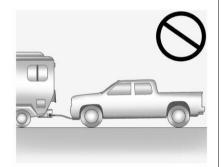
Notice: If the vehicle is towed with all four wheels on the ground, the drivetrain components could be damaged.
