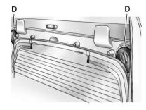
Turn both glass lock knobs (D), located at both top corners of the storage pocket, to the locked position. Push in on the corner of the rear glass to allow the lock knob to engage more easily.
