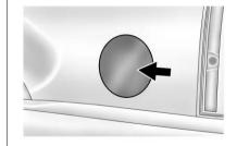
The tethered fuel cap is located behind a hinged fuel door on the driver side of the vehicle. If the vehicle has E85 fuel capability, the fuel cap will be yellow and state that E85 or gasoline can be used. See Fuel E85 (85% Ethanol) on page 9-57.
