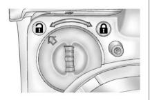
2. Hold the rear glass in place with one hand and turn the glass lock knobs, located at both top corners of the glass storage pocket, to the unlocked position.
