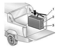
Starting with cargo panel 1, load the cargo panel with the latches facing up toward the side of the cargo box.
