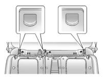
The top tether anchors are located on the back of the rear seat frame above the floor for each rear seating position. Fold down the rear seatback(s) to access the anchors. See *Rear Seats on page 3-10*. Be sure to use an anchor located on the same side of the vehicle as the seating position where the child restraint will be placed.
