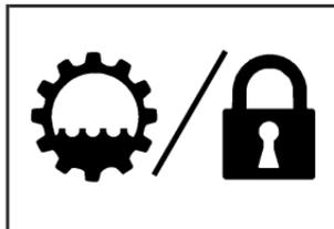
The transmission dipstick handle with this graphic is located at the rear of the engine compartment, on the passenger's side of the vehicle.
