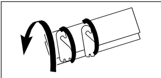
4. Take the secondary strap and wrap it around the package. Finally, attach the hooks to the webbing and place inside the top box storage compartment.
