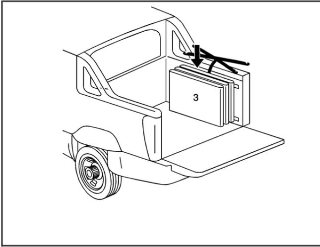
4. Store cargo panel 3 by loading the cargo panel with latches up and facing away from you.
