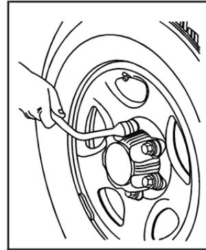
2. If the vehicle has a center cap, place the chiseled end of the wheel wrench in the slot on the wheel and gently pry the cap out.
