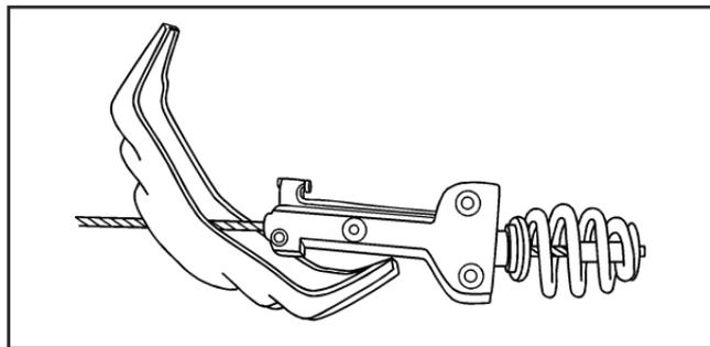
7. Tilt the tire with slack in the cable to access the tire/wheel retainer (D). Separate the retainer from the guide pin by sliding the retainer up the pin while pressing down on the latch. When the retainer is separated from the guide pin, tilt the retainer and pull it through the center of the wheel along with the cable and guide pin.
