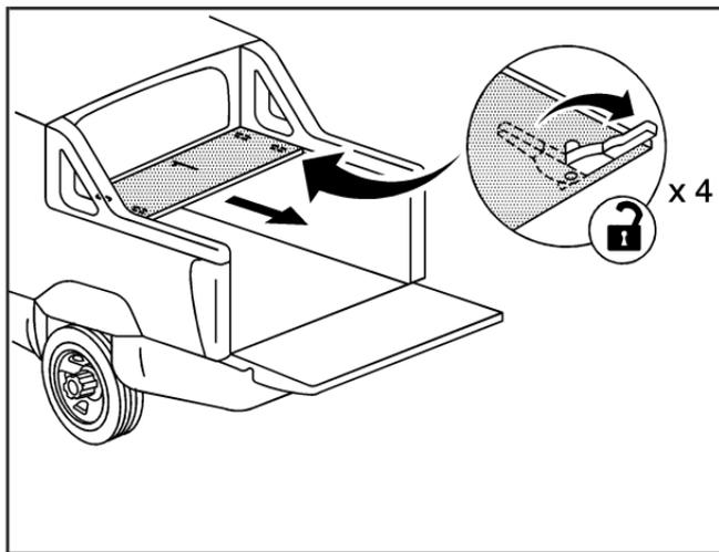
4. If cargo panel 1 needs to be removed. There are latches on both sides that need to be released.
