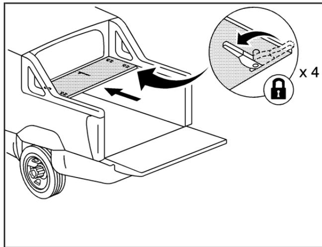
3. Push both left latches away from you to lock the latches. Remember that there are four latches total for panel 1. You should hear a click when each latch locks. Lock the remaining two right latches on panel 1.
