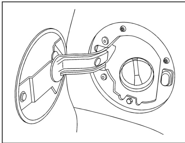
The tethered fuel cap is located behind a hinged fuel door on the driver's side of the vehicle. If the vehicle has E85 fuel capability, a yellow cap with the words "E85 or gasoline" can be seen.
