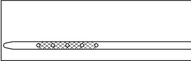
If the oil is below the cross-hatched area at the tip of the dipstick, add at least one quart/liter of the recommended oil. This section explains what kind of oil to use. For engine oil crankcase capacity, see *Capacities and Specifications on page 5-113*.
