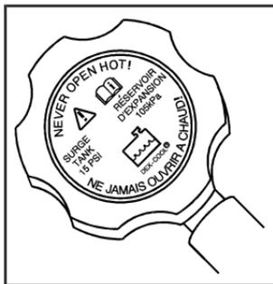
The coolant surge tank is located in the engine compartment on the passenger's side of the vehicle. See *Engine Compartment Overview* on page 5-14 for more information on location.
