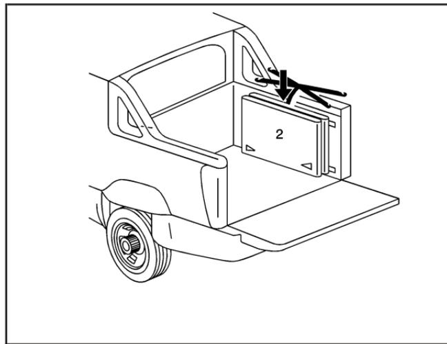
3. Store cargo panel 2 by loading the cargo panel with latches down and facing toward you.
