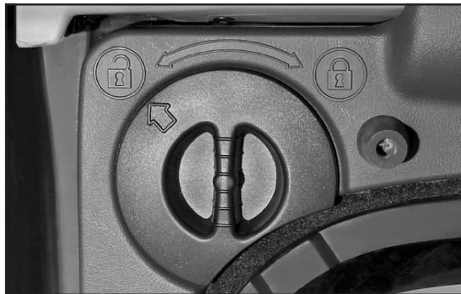
2. Hold the rear glass in place with one hand and turn the glass lock knobs, located at both top corners of the glass storage pocket, to the unlocked position.
