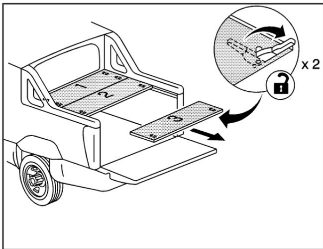
2. Remove cargo panel 3 by pulling the left and right cargo panel latches, located on the bottom of each cargo panel, forward to unlock the cargo panel latches.
