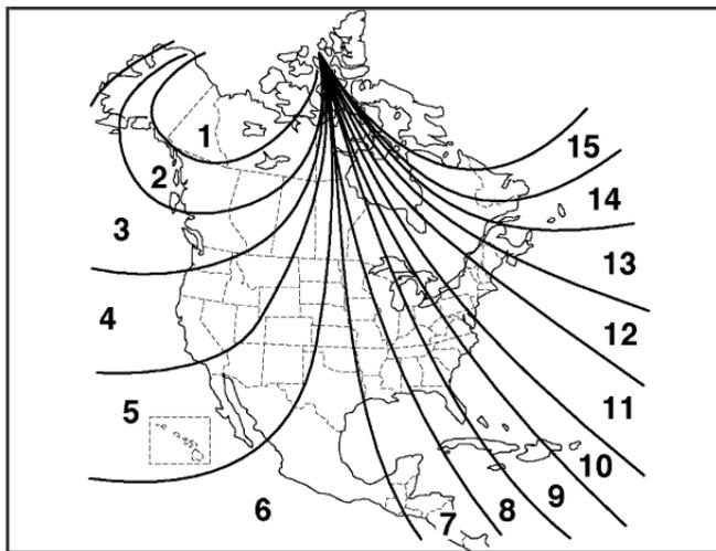
2. Press and hold the COMP button for five seconds until a zone number appears in the display.
