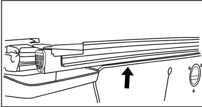
The side rail channels are located on top of both sides of the cargo area. Flush them out with clean water debris collects inside of them.
