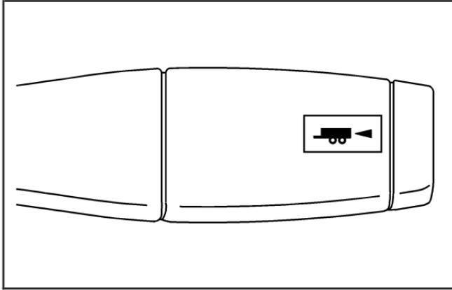
Your vehicle has a tow/haul mode. The button is located on the end of the column shift lever. Press the button to enable or disable the tow/haul mode. You can use this feature to assist when towing or hauling a heavy load. See "Tow/Haul Mode" under *Towing a Trailer on page 4-47* for more information.
