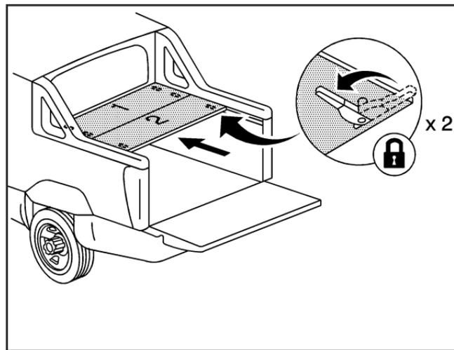
5. Push the latches away from you, starting with the left latch, to lock the panel in place. You should hear a click when each latch locks correctly.
