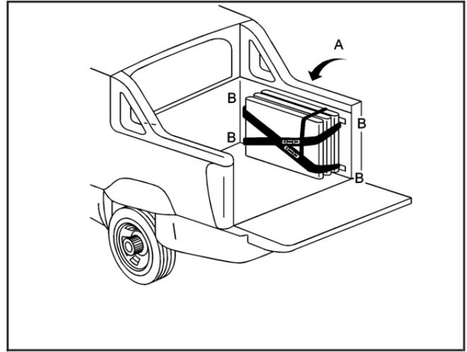
5. Place the primary straps (A) over the three cargo covers (A). Fasten the four strap clips (B).
