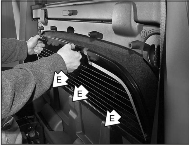
5. Load the rear glass into the storage pocket in the Midgate<sup>®</sup>, guiding the lower edge of the rear glass behind the three rear glass retaining tabs (E).
