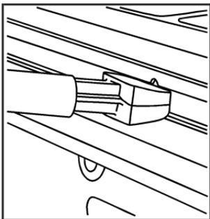
2. Remove the two bows by gently pushing them against the spring-loaded end. Set the bow aside.
