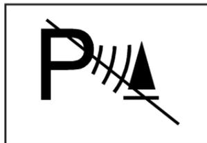
The system can be disabled by pressing the rear park aid disable button located next to the radio. The indicator light will come on to indicate that URPA is off.
