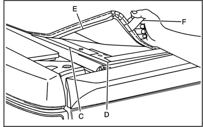
1. Starting at the rear corner of the driver's side of the vehicle, pull the loop (F) toward you and then pull up so the plastic lip (E) releases from the channel in the rear rail (D) and the side rail (C).
