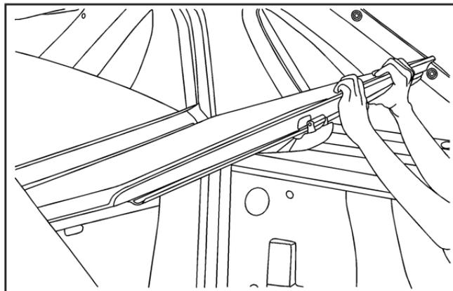
2. Starting with cargo panel 1, place the latches in the unlocked position. Place cargo panel 1 on the cargo area rails while holding the back of the cargo panel up.
