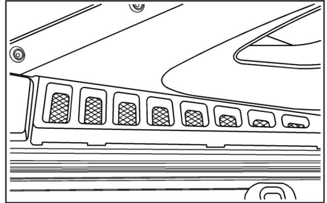
The top drain grates are located near the rear glass on both sides of the vehicle. Clean the grates and drains if there is a blockage.
