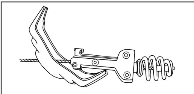
14. Tilt the tire retainer at the end of the cable and pull it through the wheel opening. Pull the tire out from under the vehicle.
