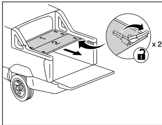
3. Pull each cargo panel up and then out from the side rails and set it aside. Remove as many cargo panels as needed.
