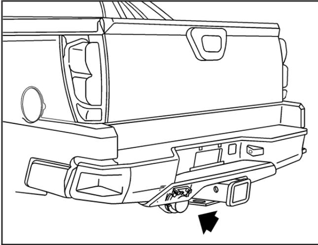
Your vehicle is equipped with the seven-wire trailer towing harness. This harness with a seven-pin universal heavy-duty trailer connector is attached to the rear bumper beam. It is located next to the integrated trailer hitch.
