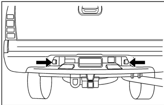
2. Turn the bulb socket counterclockwise and pull the bulb socket out of the connector.
