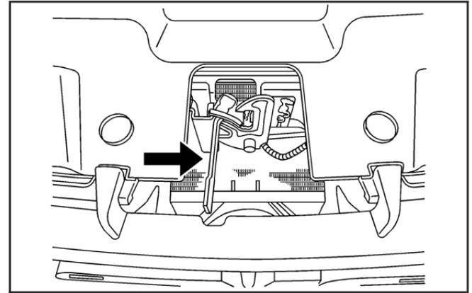
2. Then go to the front of the vehicle and locate the secondary hood release, near the center of the grille.
