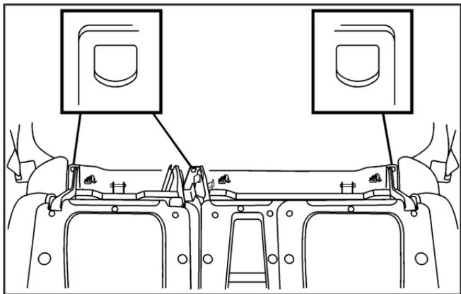
The top tether anchors are located on the back of the rear seat frame above the floor for each rear seating position. Fold down the rear seatback(s) to access the anchors. See *Rear Seat Operation* on page 1-11.
