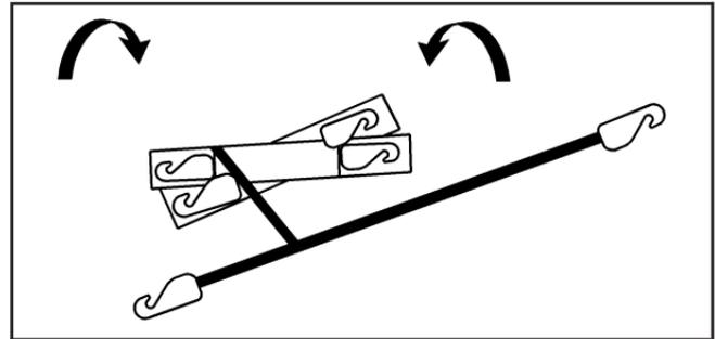
2. Fold the four primary strap ends towards the center as shown.
